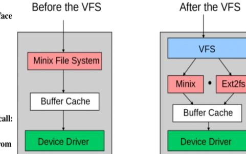
Software layer in the kernel that provides the file system interface to user space programs.
